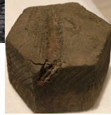
Mesquite Hexagon Exterior Blocks, Circa 1900 Mesquite blocks were once used in Texas as street pavers. Rumor has it the horses were very happy walking on end grain Mesquite!
